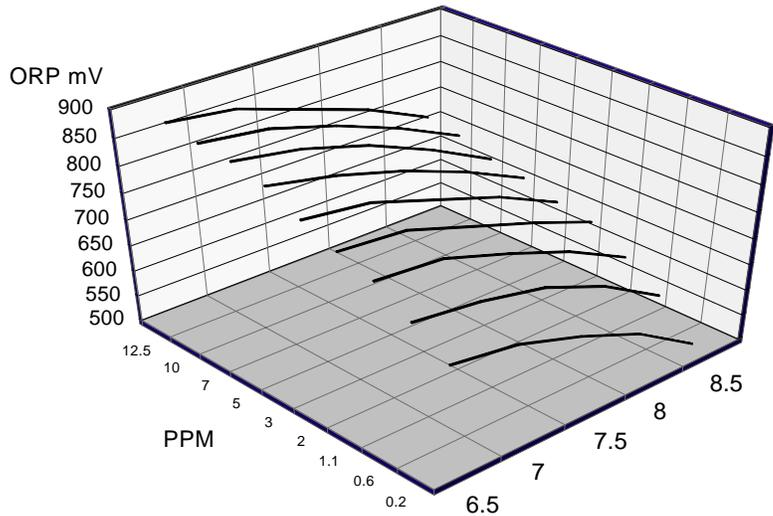
Figure 1 - Variations of ORP with PPM and pH
