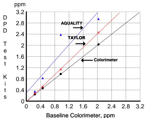
Figure 2 - Comparison of DPD Test Kits
